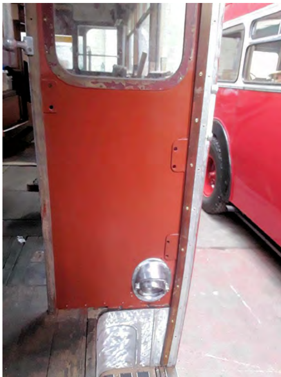
Above: The emergency light on Cardiff 262.
